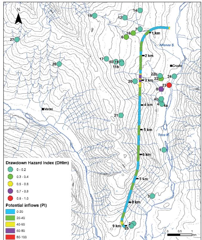
Fig. 9: Potential inflows inside the tunnel according to Dematteis method and modified Drawdown Hazard Index (DHIM) at the water point (springs and wells).
