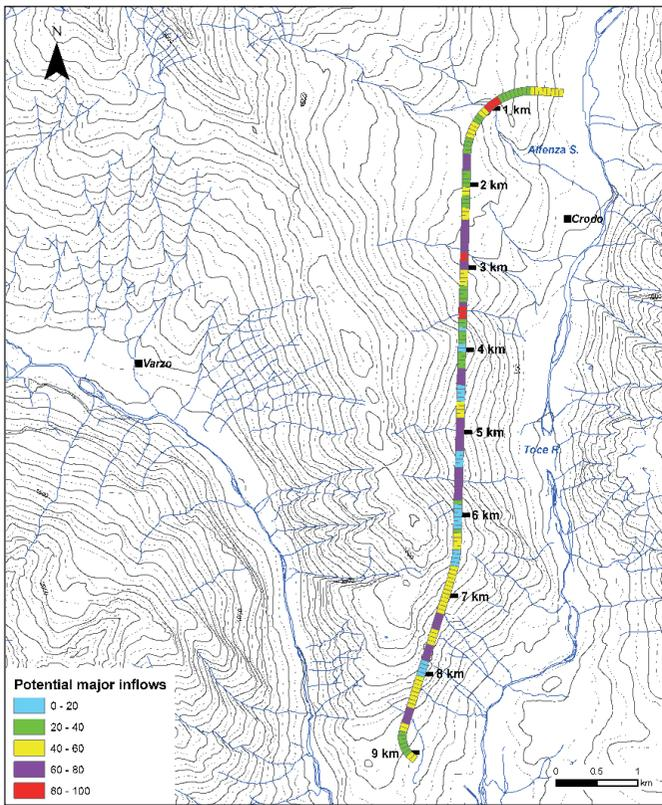
Fig. 10: Potential major inflows inside the tunnel according to Cesano method.
