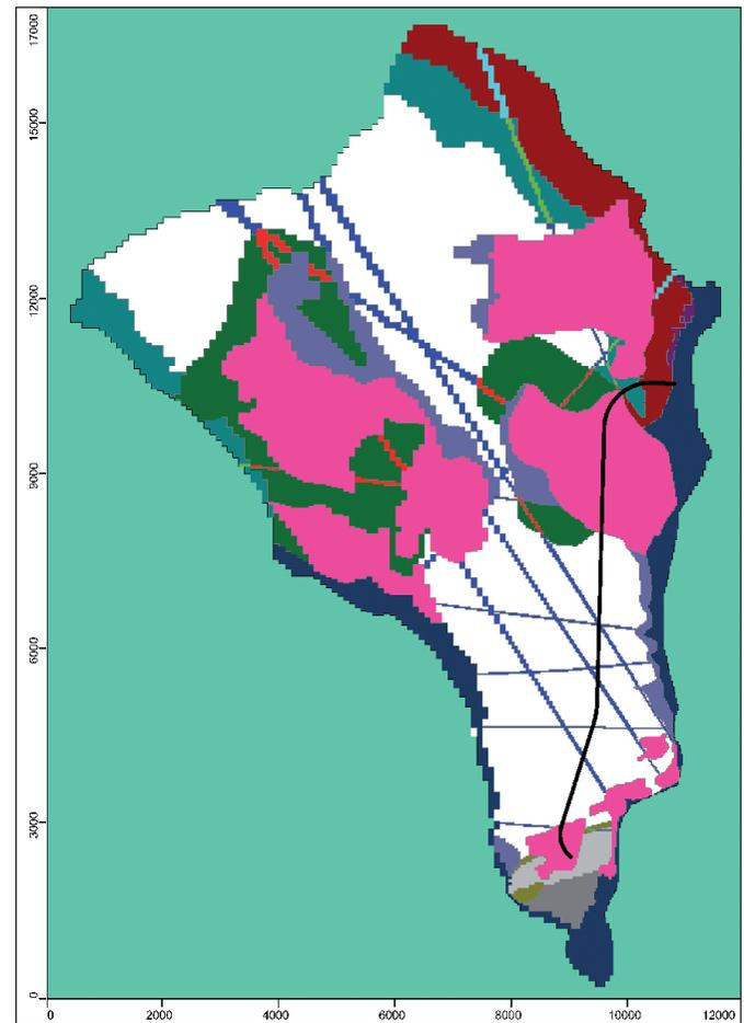
Fig. 4: Flow domain and K zones at layer 1 of the MODFLOW model. Colors corresponding to K zones according to table 3; the inactive cells are represented with the green color; coordinate axis in meters; tunnel trace in black.
