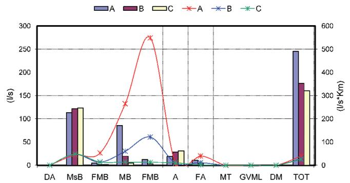
Fig.12: Total forecasted tunnel outflow (bars, left scale) and specific outflow normalized on distance (line, right scale) in relationship to lithology (DA = Quaternary fluvial deposits, MsB = Baceno Micascists, FMB = Fault zones in Baceno Micascists, MB = Baceno Metasediments, FMB = Fault zones in Baceno Metasediments, A = Antigorio Gneiss, FA = Fault zones in Antigorio Gneiss, MT = Teggiolo Metasediments, GVML = Valgrande and Monte Leone Gneiss, DM = Glacial deposits, TOT = Total).
