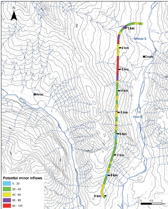
Fig.11: Potential minor inflows inside the tunnel according to Cesano method.
