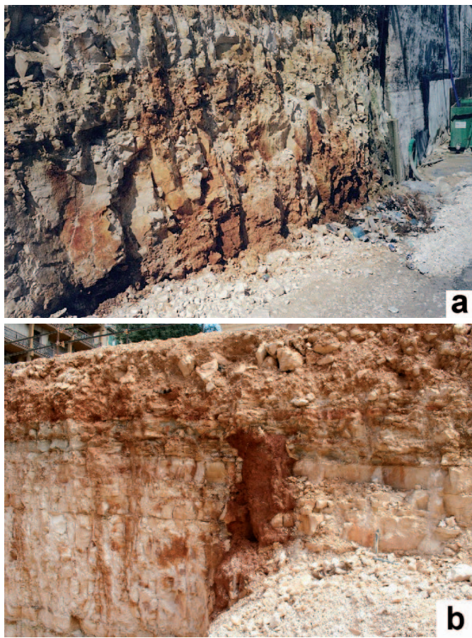
Fig. 3: Lithologic stratigraphy referred to the Cretaceous Formation recognized during the excavation for the multilevel parking in "Cesare Battisti" square - Bari.
